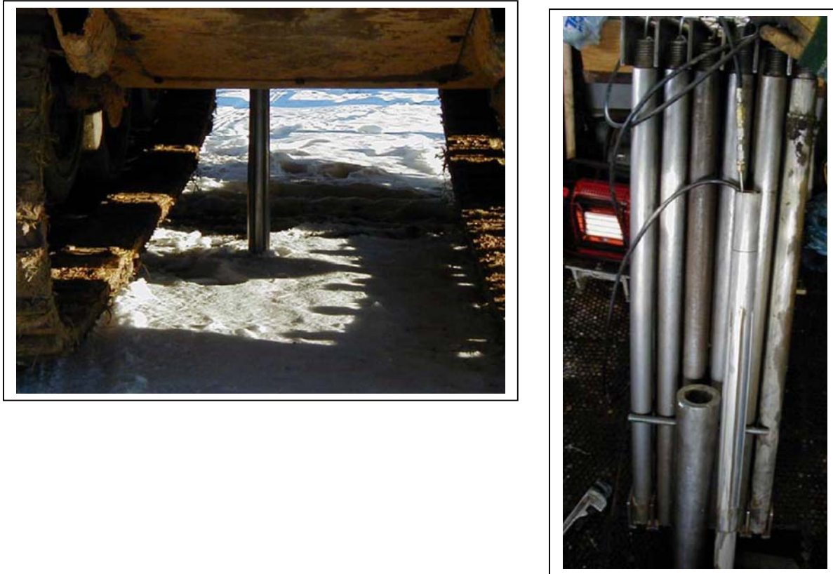
Figure 1. Left: Push-in pressuremeter being pushed into soil Right: Push-in pressuremeter showing tubing quick-connect and calibration tube
