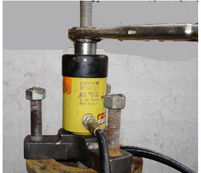
Figure 3: Rock borehole shear test piston extending upward shearing the rock
